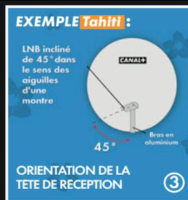
EN CONSIDERANT QUE LA PARABOLE EST UNE HORLOGE, LE CABLE QUI PART DE LA TÊTE LNB DOIT INDiquer 7H30.
