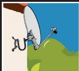
LA PARABOLE PEUT AUSSI ÊTRE INSTALLÉE SUR UN MUR SOLIDE GRÂCE AU KIT DE FIXATION FOURNI.
