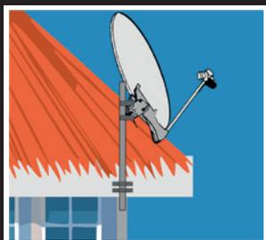
FIXEZ TOUJOURS SOLIDEMENT LA PARABOLE SUR UN MAT RIGIDE ET CYLINDRIQUE, À NIVEAU. CONTRÔLEZ CHAQUE ANNÉE QUE LES FIXATIONS SOIENT BIEN VISSÉES AU SUPPORT.
